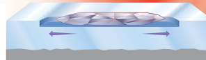
Flat or crystal-shaped ice melters melt across the ice, so they penetrate and break the ice’s bond with the pavement more slowly.
